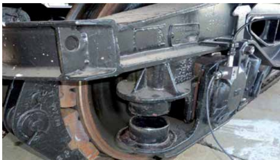
Fig. 2. Freight car bogie with removed springs
